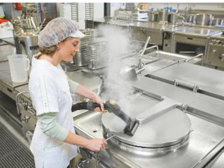
Industrial steam cleaners are convenient because the cleaning parameters can be adjusted directly on the gun. In addition, the dissolved dirt and debris are immediately vacuumed up.
