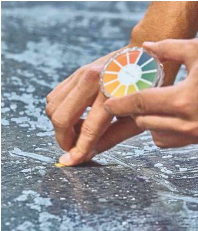
The pH value can be conveniently checked with an indicator strip.
